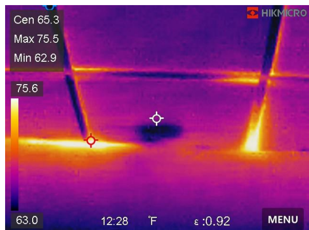
Thermal imaging confirming leak is active
